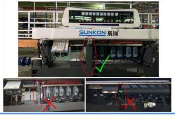
The front beam is hanging with 7 motors. A strong pillar in middle to make sure front beam indeformable even with heavy bearing.
