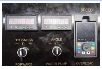
Digital display to show the glass thickness and angle. Speed is easy frequency control.
