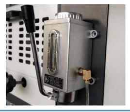
Lubricating system with oil pump to keep spindles always in lubrication state, better for maintenance.
