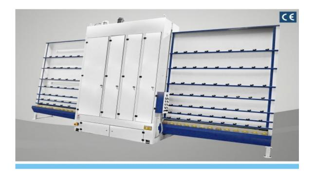
MODEL : YG2.0LCV MAKE : YG /CHINA Max. size of glass : 2000mm Min. size : 350x350mm ✓ Glass thickness : 3-19mm ✓ Speed : 1.9-3m/min **Brush roller** : 3 pairs Power : 15kw
